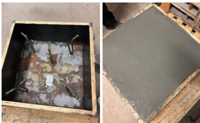
Figure 2. A block of the castable solution was cast and then used as the door of the test furnace.
