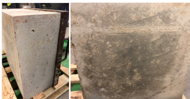
Figure 3. No cracks could be found in the cast block after the kiln heating up procedure.
