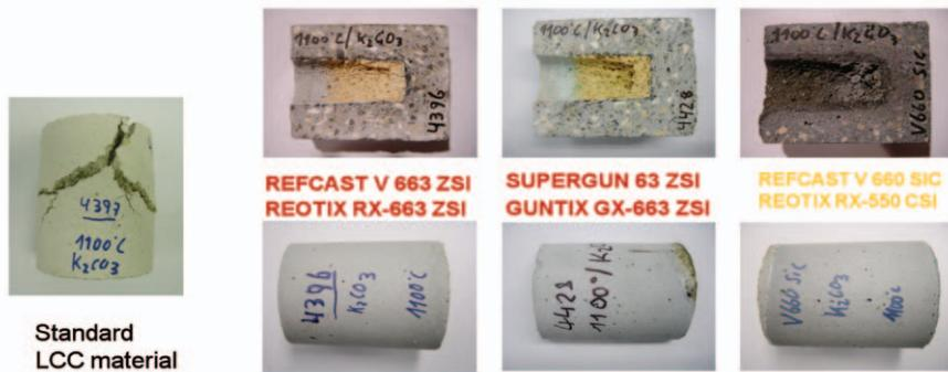
Figure 1. Alkali bursting test (5 h at 1100 °C with K<sub>2</sub>CO<sub>3</sub>)
